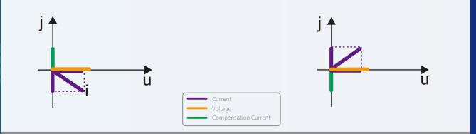
Because most of the electrical equipment is inductive load, the power factor is obviously less than 1 during operation, a large amount of reactive power needs to be taken from the grid. Therefore, in order to improve the power factor of the grid, it must compensate the reactive power in the grid.
